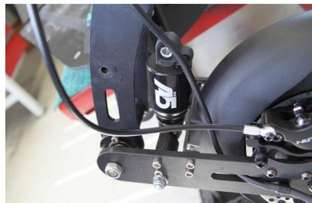
2. push the shock absorber a little back, to fill air better in the filler neck to pump. Not more than 150psi or 10 bar.
