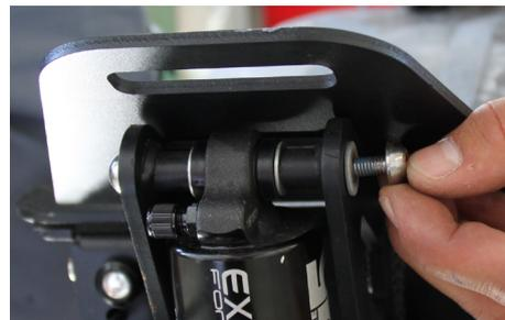
Slide the screw and washers back in and tighten the screw again.
