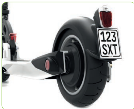
Brushless hub motor in rear wheel / Auto Power Off function
